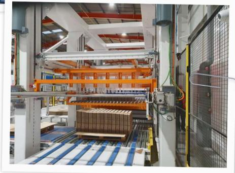
Bottlenecks in production – often converting machines are not run at full capacity due to barriers in materials handling. Die-cutters are being slowed down to keep pace with existing separators or palletisers. These constraints can be overcome by Pegasus with these features:
