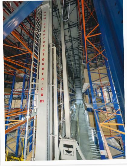
system in the UK alongside partner DF. This system gave SAICA 900,000 sqm of board storage in Work In Progress in a compact 18m x 50m x 15m space. A regular conveyor system would have provided about 200,000 sqm of space. This meant that SAICA could deckle the corrugator by
